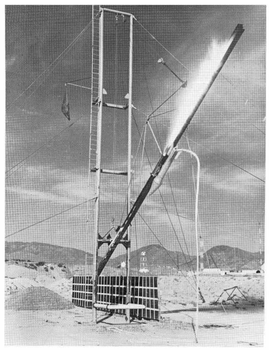
NOBODY GOOFED—an artist changed the shape of this test vehicle, but not the direction. Environmental test engineers have been launching rocket-powered vehicles downward for more than two years. The tests are conducted to subject components and systems to impact environments.
